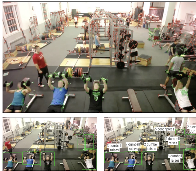
Figure 1: GymCam is a camera-based exercise tracking system that uses optical flow to track, detect and recognize activities for 100s of users at the same time.
